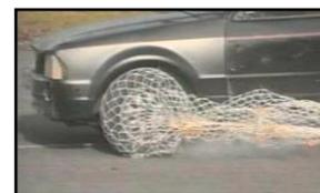
Vehicle Lightweight Arresting Device M2 Net
