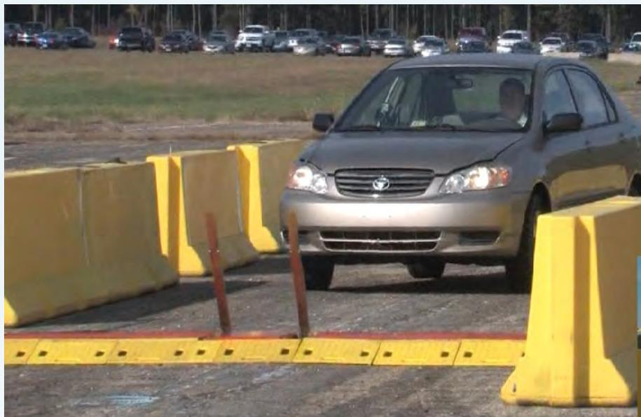
*A vehicle approaches the Pre-Emplaced Vehicle Stopper.*
